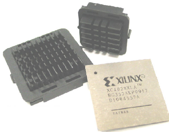
Figure 3-12: Enhanced BGA with Low Profile Retainer Type Passive Heatsinks
