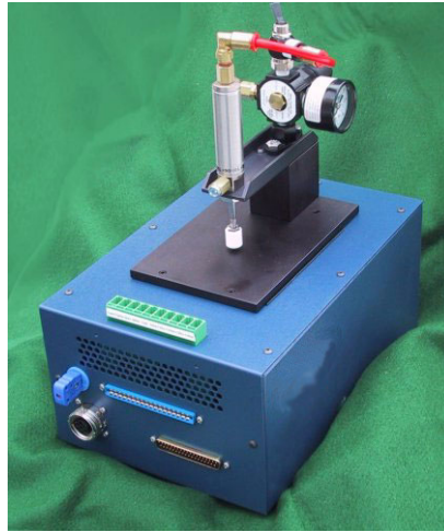
Figure 3-3: Theta JC Measurement Setup
