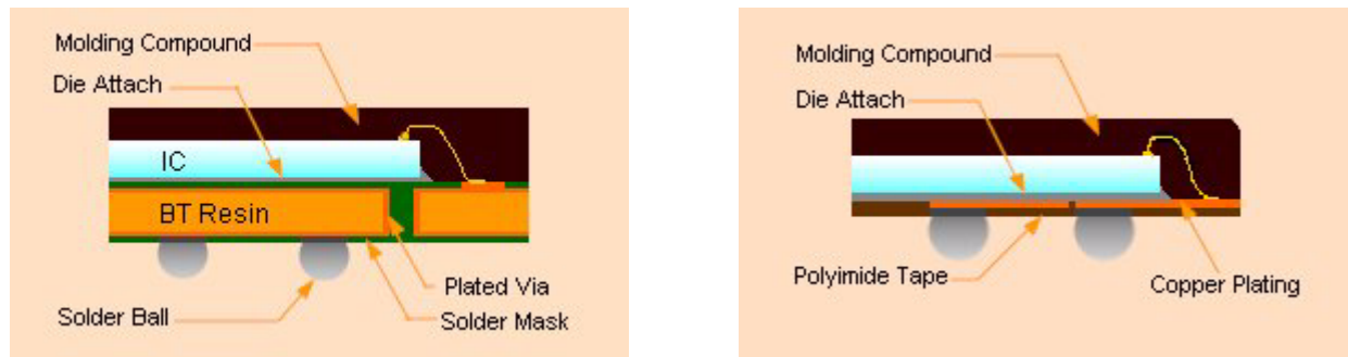
Figure 1-7: Rigid BT-based Substrate Chip Scale Packages, left; Flex-Based Tape Substrate, right
