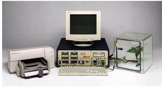
Figure 3-4: Theta JA Measurement Setup
